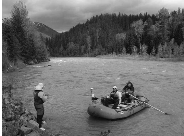
Figure 1. Scientists Chris Gotschalk, Diego Tonolla, and Mark Lorang calibrate an Acoustic Doppler Profiler, before a series of floats, down the Middle Fork Flathead River. Photo by Charles Nichols.
