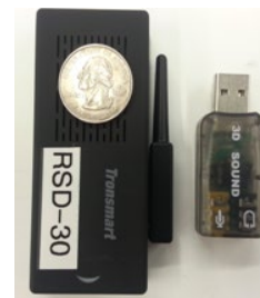
Figure 3. Android fixed RSD proof-of-concept showing processor and audio CODEC (left-hand)
