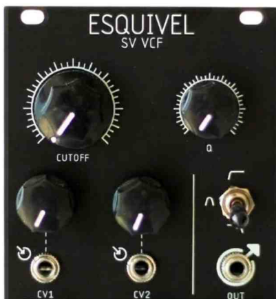
Figure 3. Bocuma "Esquivel" State-Variable Filter Module Esquivel Front Panels. Esquivel faceplates V1 and V2. Bocuma. www.bocuma.mx/product/esquivel
