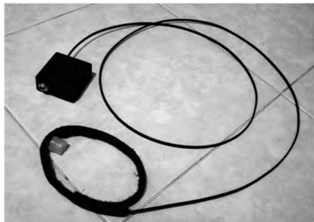
Figure 2. Xth Sense wearable MMG sensor prototype
